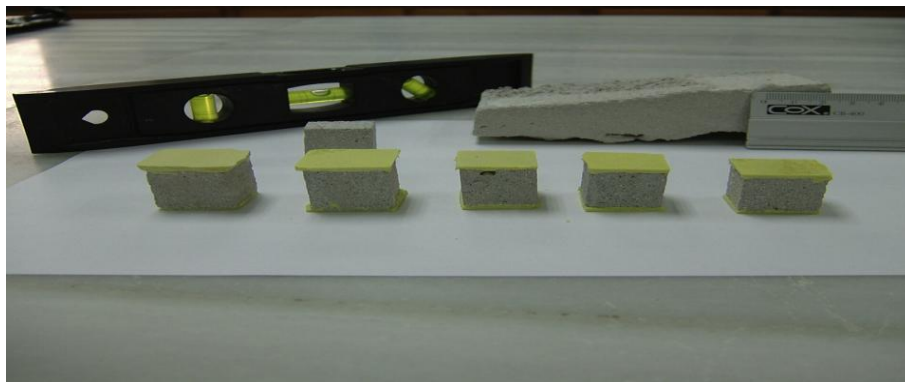
Figure (1)- Cubic micro cores of mortar capped with sulfur used in (Alejandro) experiment [18]
