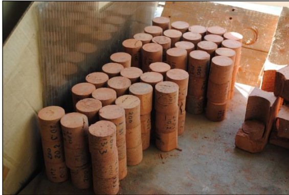
Figure 6. Part-drilled core samples
