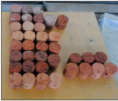
Figure 2 The cores selected from the arch
